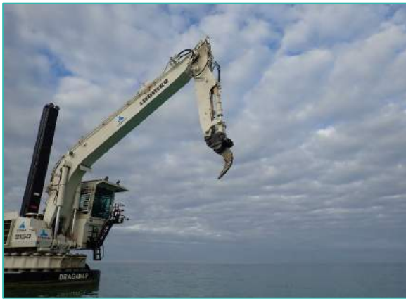
Figure 19: Ripper tooth on dipper pontoon (photo courtesy: NEREIS Environnement).
