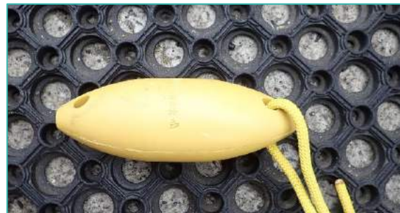
Figure 17: AQUAmark® 210 (AQUATEC) acoustic deterrent used on fishing gear (photo courtesy: NEREIS Environnement).
