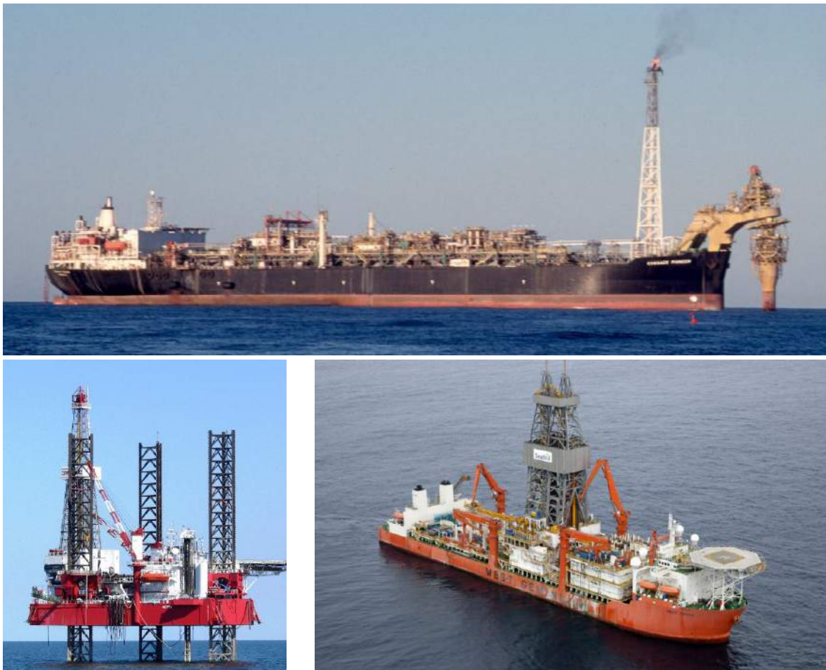
Figure 13: Cossack Pioneer mobile rig of FPSO (Floating Production Storage and Offloading) type [60], Astra jack-up rig (photo courtesy: EDC Ltd.) and West Gemini drillship (photo courtesy: Thierry Gonzalez/TOTAL).
