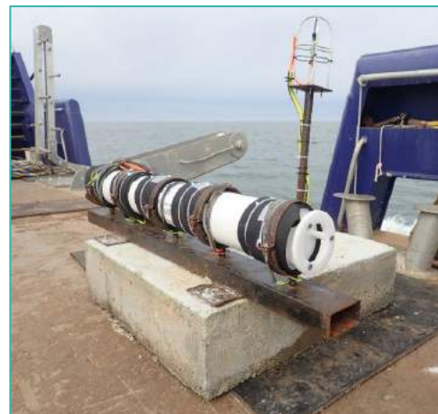
Figure 7: Autonomous acoustic recorder (OSEAN) equipped with a hydrophone and positioned on a mooring post before immersion (photo courtesy: NEREIS Environnement).
