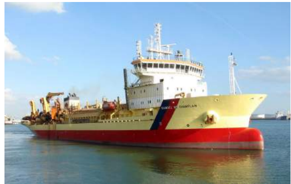
Figure 18: The Samuel de Champlain suction dredger in action (GIE Dragages-Ports, photo courtesy: Fabien Montreuil).
