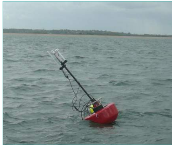
Figure 8: Autonomous floating acoustic buoy (RTSys - photo courtesy: NEREIS Environnement).
