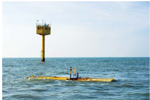
NEMOS WEC 2019 prototype floater deployed close to the NEMOS research tower (source: NEMOS, Cornelius Weikert)
