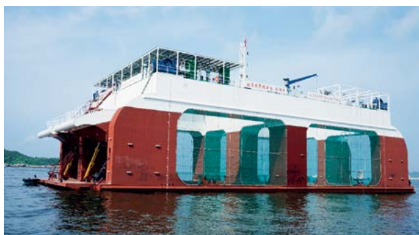
Wave energy aquaculture cage “Penghu” in sea test (Length 66m, Depth 28m, and Height 16m, 120kW Wave energy, 10,000m 3 aquaculture space).
