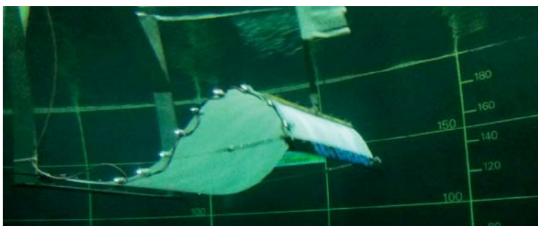
1/20 scale membrane prototype of the Eel tidal converter tested in the Ifremer flume of Boulogne/mer
