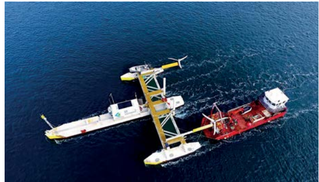
PLAT-I 4.63 platform with two turbine arms in maintenance position (source: SCHOTTEL HYDRO)
