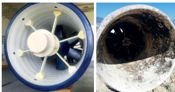
Equipment tested by the CEMIE-Oceano showing bio-incrustation after only 50 days at sea
