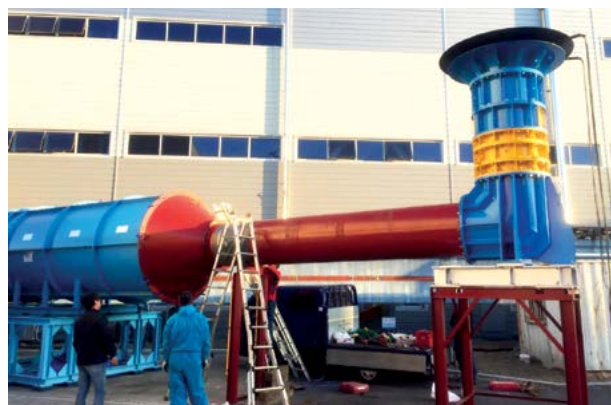
Performance test on prototype of impulse turbine with generator (Courtesy: KRISO)
