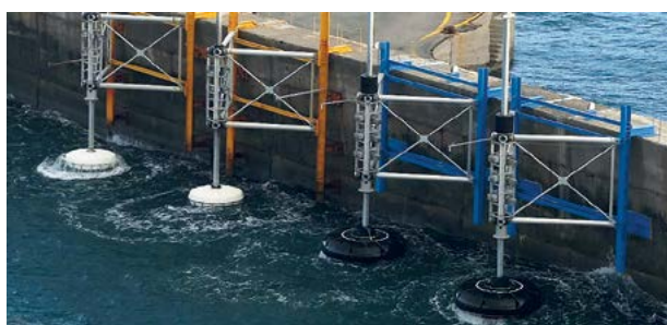
Third (left) and fourth generation SINN Power WECs at the port of Heraklion, Greece (source: SINN Power)
