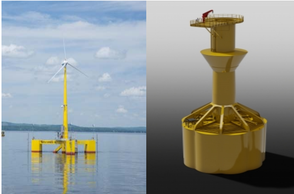
Figure 10. Representative substructures proposed in DOE's ATD program Sources: University of Maine (left); LEEDCo (right)
