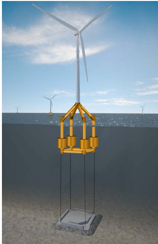
Figure B10. Illustration of the GICON-SOF floating offshore wind turbine system under development in Germany
