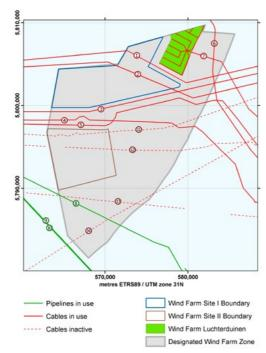
Two inactive cables (11 and 12) cross HKZWFS II. As they are no longer in use, they do not require maintenance zones and they are assumed not to affect the effective area. An overview of all the existing infrastructure can be found in the GIS files at: *offshorewind.rvo.nl*.
