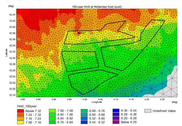
Figure 40 Significant wave height with a 100-year return period at the Hollandse Kust (zuid) (left) including the output location
