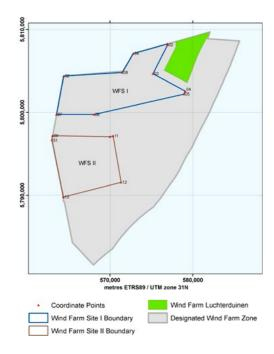
The water depth ranges from 18.1 m to 27.8 m with respect to Lowest Astronomical Tide (LAT) across HKZWFS I and 18.8 m to 26.6 m LAT across HKZWFS II. The bathymetry of HKZWFS I and II is shown in Figure 3d.
