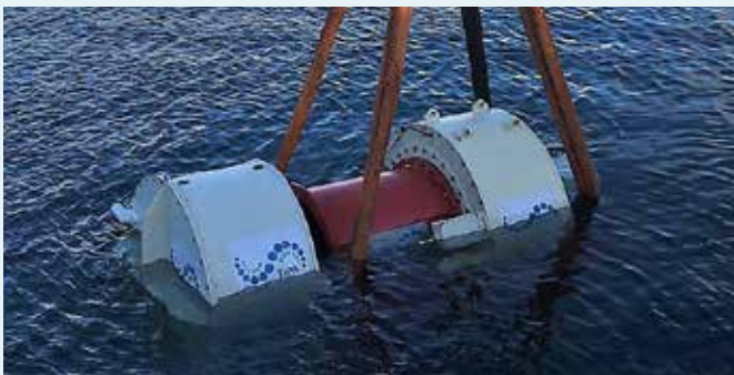
Figure 13. Deployment of TiPA PTO for subsea testing.
