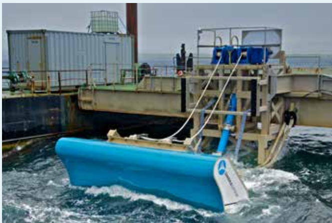
Figure 18. The EMERGE project has developed an innovative ballscrew-based PTO reaching TRL7.
